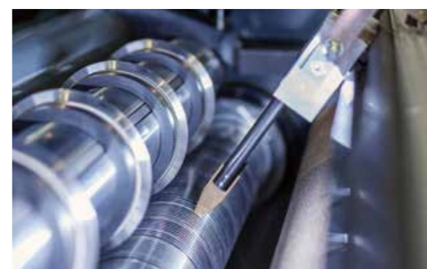
Positioning aid Time-saving and precise alignment for bottom knife and razor blade grooved bushes.
