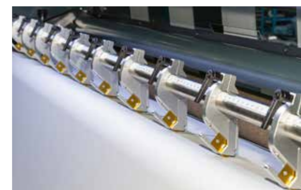
Razor blade cut Reasonable and good. Optionally as groove or mirror cut.
